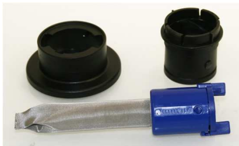
Urea filler neck to be welded with hot blade, bayonet connection \varnothing 40 , with 40 micron filter, with neodymium magnet
