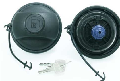
Locking diesel tank cap, bayonet connection \varnothing 60 , vented with equa valve, with external plastic cord
